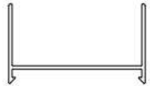
Semi-FL Slider Wall Jamb E-WJSFL (E-210)
