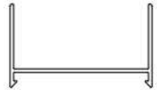
Semi-FL Slider Wall Jamb E-WJSFL (E-210)
