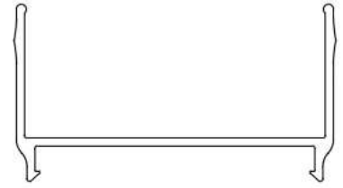
Framed Slider Wall Jamb E-FSWJ (E-110)
